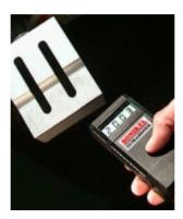
Ultrasonic Frequency Meter provided by Sonikel Ultrasonics, is used to measure the horn frequency in industrial applications. This measurement is performed to analyze the efficiency of the ultrasonic system or automation solution. The measurement is realized without touching the system. Ultrasonic Frequency Meter is pocket-size so it is commonly preferred by technical people at factories.
